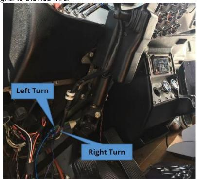
4. **2005-2007 387:** Turn signal connections are found in the harness coming out of the steering wheel. Using Posi-Taps, connect the Left Turn signal to the Green wire and the Right Turn signal to the Red wire.
