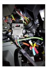
3. **2001-2007 379:** The J1708 connections will be found on the back of the diagnostics port. They are a twisted pair and will need to be tested for voltage to confirm.
