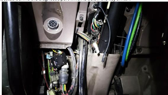
3. **2014-2014 579:** The CAN bus coupler is attached to the J1939 backbone. This is located in the area directly above the fuse panel, near where the driver's left knee would be.
