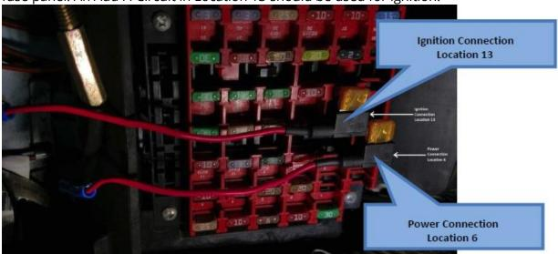
3. **2001-2007 379:** Connections are made with Add-A-Circuits and connected to the fuse panel by the drivers left foot.
